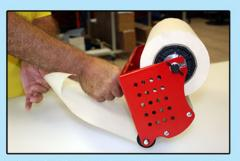
Lift the Pro-Roll Tape Applicator with handle in one hand. Pull transfer tape down and under the rubber roller with the other hand. Pull between 9-12" of transfer tape beyond the black rubber roller. Keep tape tight against black roller.
