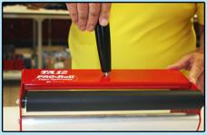
Attach the black handle (loose inside the box) by screwing it directly into the Pro-Roll Tape Applicator Tool.
