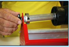
Unscrew thumbscrews on both sides of the Pro-Roll Tape Applicator Tool. Remove mounting rod from Pro-Roll Tape Applicator Tool.
