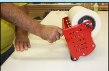
Continue to keep application tape tight against the black rubber roller. Lower the Pro-Roll Application Tape Tool allowing the rubber roller to now touch the table directly in front of the graphics needing application tape applied to them.
