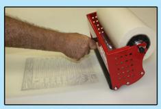
Simply tilt the Pro-Roll Tape Applicator back using the handle, lifting the application tape off of the table. Push the Pro-Roll Tape Application Tool across your graphics. Do not apply pressure downward. Let the Pro-Roll Tape Applicator Tool do all the work.
