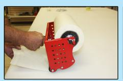
Lower your hand holding the Pro-Roll Tape Applicator Tool down onto the table so that the application tape roll is resting on the table.
