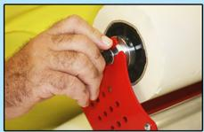
Tighten both black thumbscrews tightly to lock rod onto the Pro-Roll Tape Applicator Tool.
