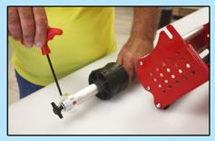
Losen the screw in the locking collar with the "T" Allen wrench (included) and remove tape core caps from the mounting rod.
