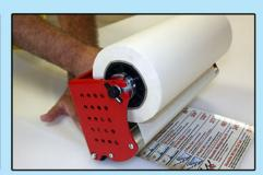
Be sure you have aligned your tape with your graphics and begin smoothing out the 9-12" of application tape onto the table to hold it in place
