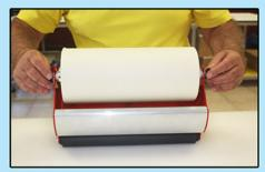
Place rod with application tape locked-on, back into the slots on the side of the Pro-Roll Tape Applicator Tool. Be sure application tape back (non-adhesive side) rolls against the black rubber roller.
